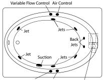
System Control Air Control Std. Pump Location
