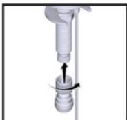
**STEP 2** – Thread on adapter fitting to the shank.
