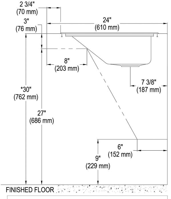
\*NOTE: ALTERING THIS DIMENSION COULD CAUSE SINK TO BECOME NON-ADA COMPLIANT
