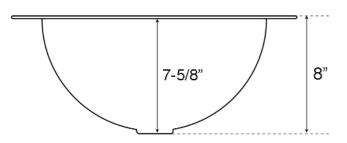
Dimensions of fixture are nominal and may vary within the range of tolerances established by ASME Standard A112.19.2. Dimensions and specifications subject to change without notice.
